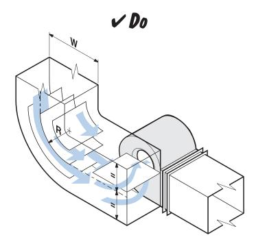
Splitters at the inlet help prevent spinning flow. Turning vanes, where R/W<1.0 improves uniformity of flow approaching the fan inlet.
