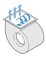
To determine the system resistance the discharge losses have to be added before selecting the fan.
