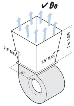
With a correctly designed discharge diffuser the pressure recovery in the diffuser will reduce the system total pressure.
