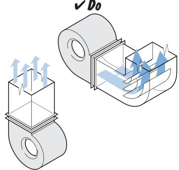
Improved discharge arrangement with radiused bends and splitters or different fan mounting position will reduce system losses
