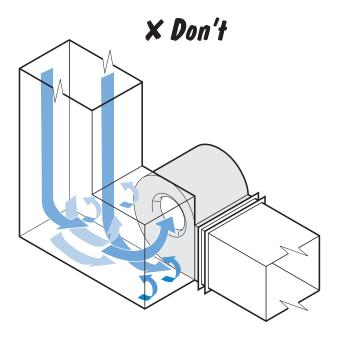
A poorly designed inlet box can generate spinning of the air which can reduce performance by around 25%.
