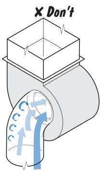
Eccentric air distribution at fan inlet diminishes fan performance by up to 45% because the main flow is accelerated through an effectively smaller duct area on one side while turbulence and high intensity pressure fluctuations occur on the other. Noise level is also increased.
