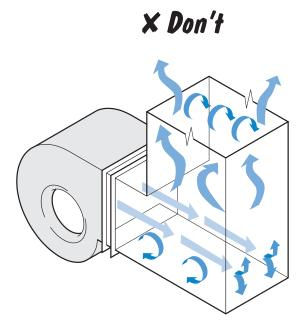
Air moves faster at the outside of the fan housing and is not evened out before striking the abrupt bend. A very high pressure loss results.
